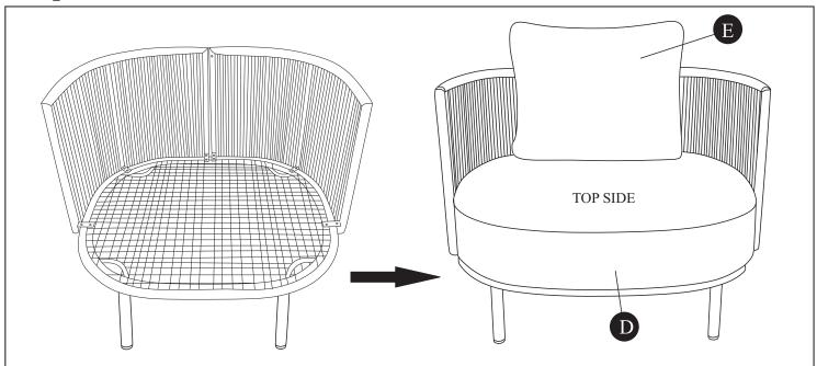
Turn assembly right side up. Place Seat Cushion (D) and Back Cushion (E) onto assembly as shown. Note the Cushion are directional and should be oriented correctly.
