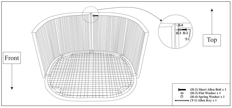
Connect Right Arm (B) and Left Arm (C) with Short Allen Bolt (H-2), Spring Washers (H-4) and Flat Washers (H-3) and stacking the hardware in the order as shown. Engage all hardware by hand, then tighten them using the Allen Key (T-1). DO NOT OVER TIGHTEN.
