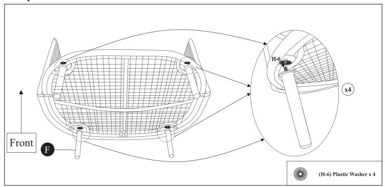
Turn on the assembly on its back onto a clean, non-marring surface. Align bolts on Legs (F) and Plastic Washers (H-6) with receiving holes underside as shown.
